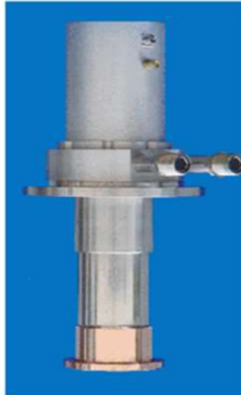
Gifford Mac-Mahon Cryomech AL 600 cold head Cooling power: 510 W @ 70 K Input power: 13 kW
