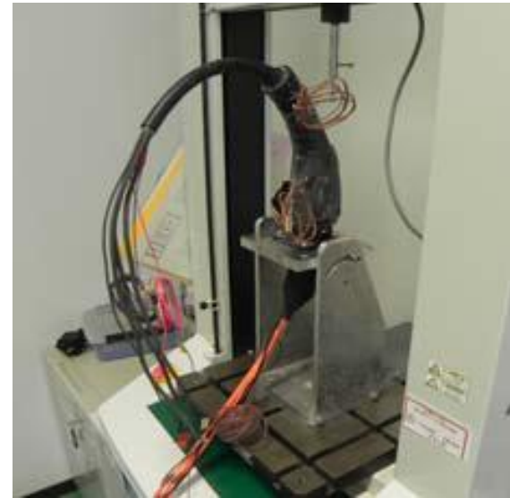
REMA Connector / Yazaki Inlet Insertion Force Measurement
