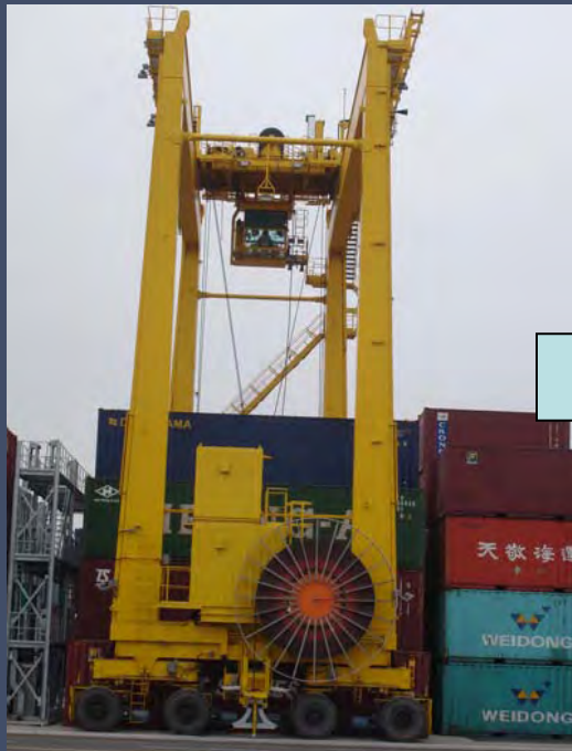
The Existing Solution: Cable Reel onboard
