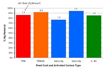
Activated carbon produced on site using pulverized coals offers mercury removal efficiencies comparable to those of commercial (Darco) sorbents.
