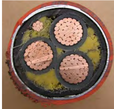
Natural XLPE insulation Cable Length: 3 ½ ft – 14 ft
