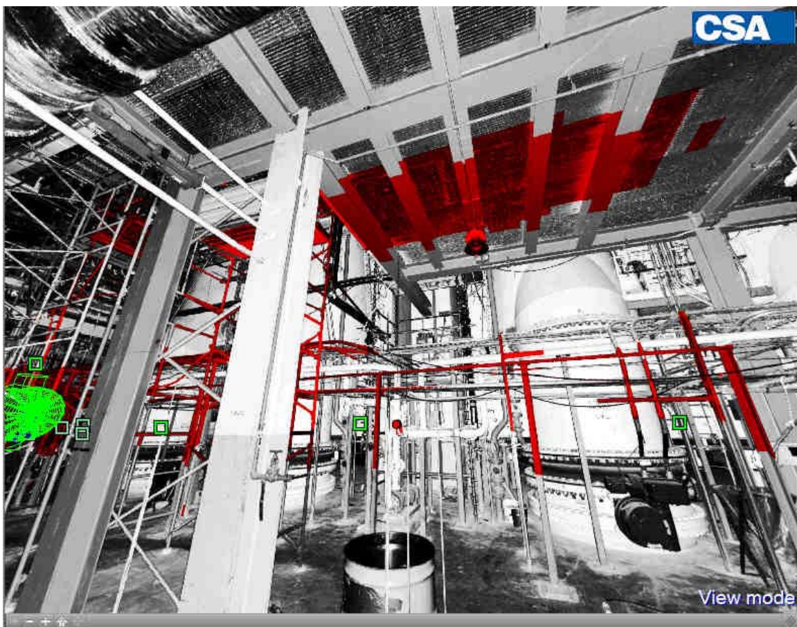
Example of Interferences within a Removal Sequence (Interferences Are Marked in Red)
