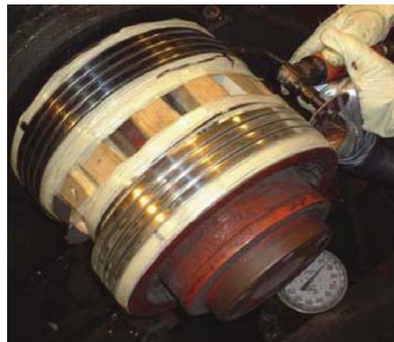
Figure 1: Recutting a worn-out helical groove (top)
