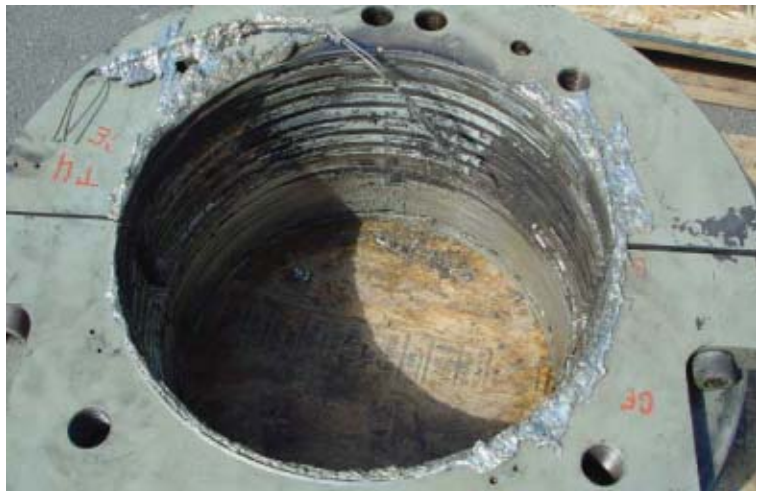
Damage to a 20+ -inch turbine bearing caused by loss of lube pumps at coal-fired power plant. Photo, Quadna.
