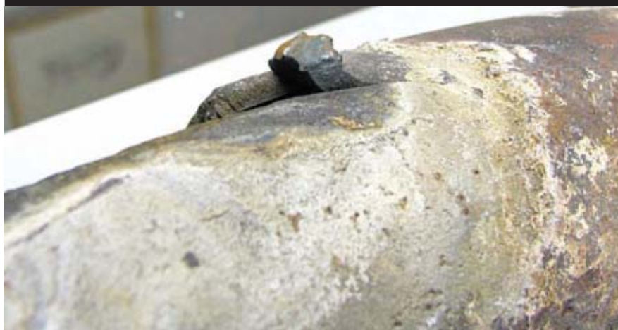
FIGURE 1 HYDROGEN DAMAGE FAILURE OF A WATERWALL TUBE. NOTE THE THICK-LIPPED FRACTURE WITH LITTLE NOTICEABLE METAL LOSS.
