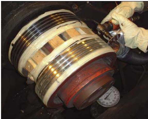
Figure 1. Recutting a worn-out helical groove.
