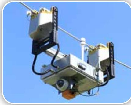
*Ti, a transmission line inspection robot, can traverse 60 miles (96.6 km) of line at least twice a year, collecting high-fidelity information that utilities can act on in real time.*
