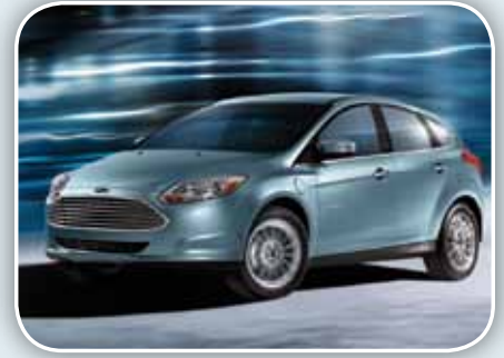
Ford plans to release the battery electric version of the Ford Focus in late 2011. The Focus Electric is powered by a lithium ion battery that can recharge from either 120 or 240 volts. Using the wall-mounted 240-volt charger can completely recharge the battery in as little as 3–4 hours. Photo courtesy of Ford.
