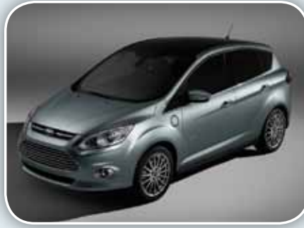
The Ford C-Max Energi is a plug-in hybrid electric vehicle that will be available in 2012. It relies on its battery at lower speeds and for stop-and-go driving. At higher speeds, the battery and gasoline engine work together to power the vehicle. Photo courtesy of Ford.
