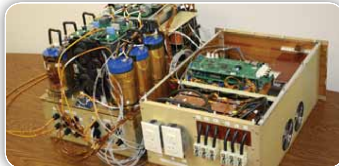
This 2.4-kV IUT prototype was tested in EPRI laboratories in 2011.
