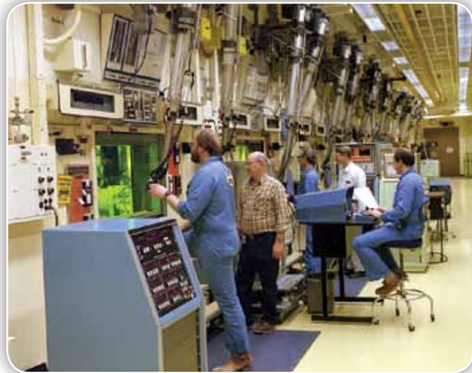
Testing of Zircaloy channels for hydrogen absorption must currently be carried out in a heavily shielded hot cell facility at great expense.
