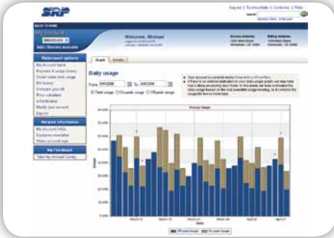
SRP's time-of-use plan allows customers to monitor their on-peak electricity use (brown bars) through a secure Web page.
