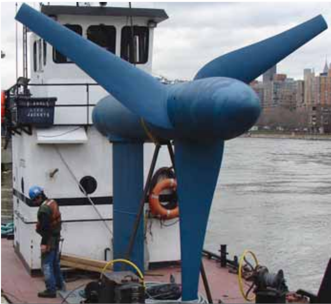
Tidal In-Stream Energy Conversion (TISEC) has been studied favorably for application at seven promising sites in North America. Verdant Power's Free-Flow turbine is shown being transported for installation in New York's East River in late 2006. (photo: Kris Unger/Verdant Power, Inc.)
