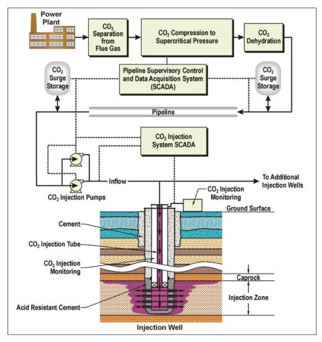
Future CCS systems will have to integrate CO<sub>2</sub> capture at the power plant with transport, geologic injection, and storage monitoring technologies in a seamless whole on a very large scale. While most of the individual components have been demonstrated in specific applications, experience with integrated end-to-end systems is extremely limited, and large-scale demos for such systems are needed. (Source: Battelle, Joint Global Change Research Institute)
