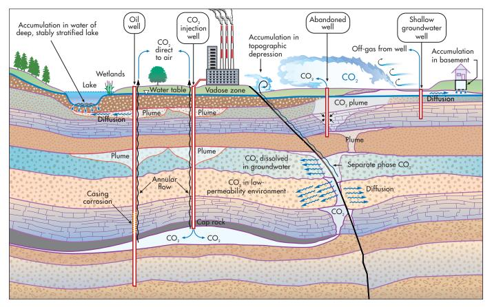
Properly sited, engineered, and managed geological reservoirs are expected to retain stored CO<sub>2</sub> for hundreds to thousands of years. However, effective monitoring systems will have to consider possible underground CO<sub>2</sub> migration paths through soils and groundwater and likely escape routes, including seismic fissures, abandoned water wells, and the injection wells themselves.
